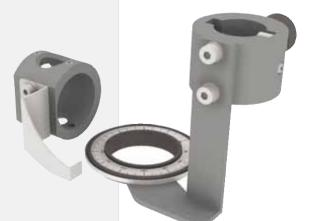
For the common rail injectors, manufacturers are specifying both torque and angle settings. With this gauge, Diesel Injection Specialists can meet the demands of the new specifications: to tighten the nuts a specified number of degrees after initial torque is set. The gauge is composed by two elements: the easy-to-read circular gauge to be installed on 10019-K, 10019-KA, 10019-KD and the indicator to be installed on the dynamometric wrench.
