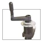
Rotate the graduated disk until the zero angle position corresponds to the arrow index.
